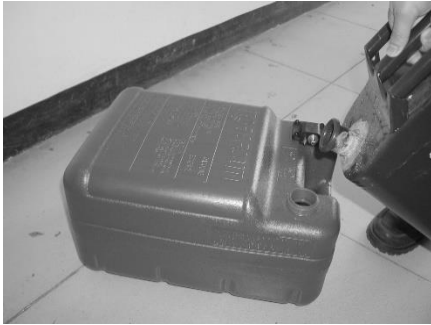
External fuel tank
